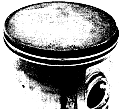
30:1 Reducing the fuel's oil content caused heavy scuffing, more varnish and a 12 percent power loss.
